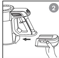
2. Press the release button to disconnect the battery pack from the main body [3].
