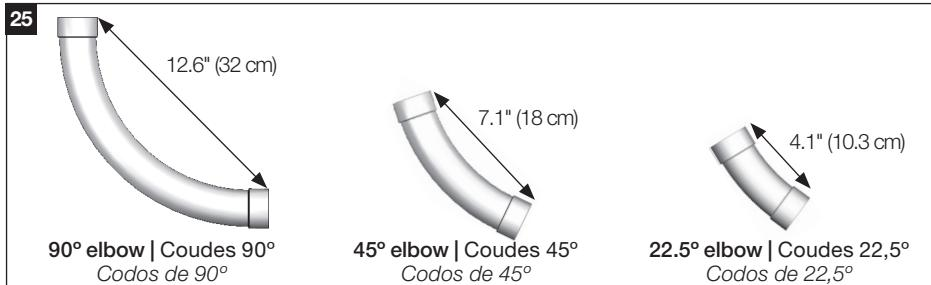
The more 90's used the more force is needed to pull the hose out of the valve. Try not to use more than four 90's for each valve.
